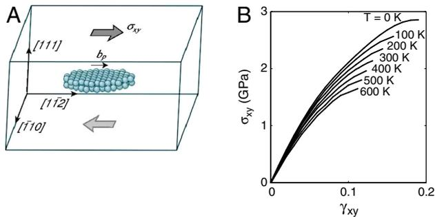
**Fig. 1.** (A) Schematics of the simulation cell. The spheres represent atoms enclosed by the critical nucleus of a Shockley partial dislocation loop. (B) Shear stress–strain curves of the Cu perfect crystal (before dislocation nucleation) at different temperatures.
