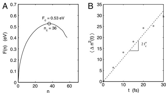
**Fig. 2.** (A) Free energy of dislocation loop during homogeneous nucleation at  $T = 300$  K,  $\sigma_{xy} = 2.16$  GPa ( $\gamma_{xy} = 0.135$ ) from umbrella sampling. (B) Size fluctuation of critical nuclei from MD simulations.
