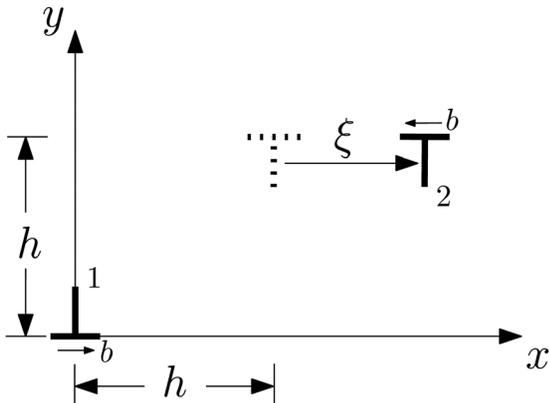
FIG. 2. An isolated dipole gliding in the  $x$ -direction. Dislocation 2 is displaced by an amount  $\xi$  away from its equilibrium position  $(h, h)$ , assuming that dislocation 1 is fixed at the origin.
