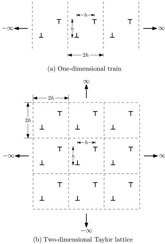
FIG. 1. Relaxed state of infinite dipole structures.
