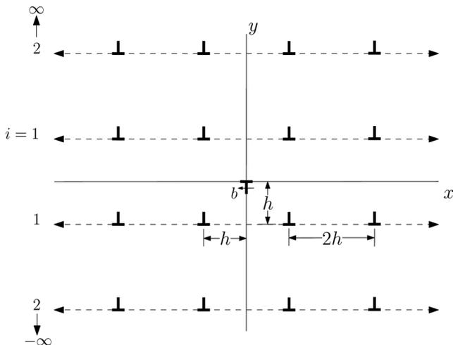
FIG. 6. Single dislocation acted on by an infinite lattice of oppositely signed dislocation walls.
