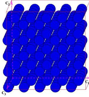
Figure 2: A perfect BCC molybdenum crystal.  $\mathbf{c}_1 = 5[100]$ ,  $\mathbf{c}_2 = 5[010]$ , and  $\mathbf{c}_3 = 5[001]$  are the periodicity vectors.
